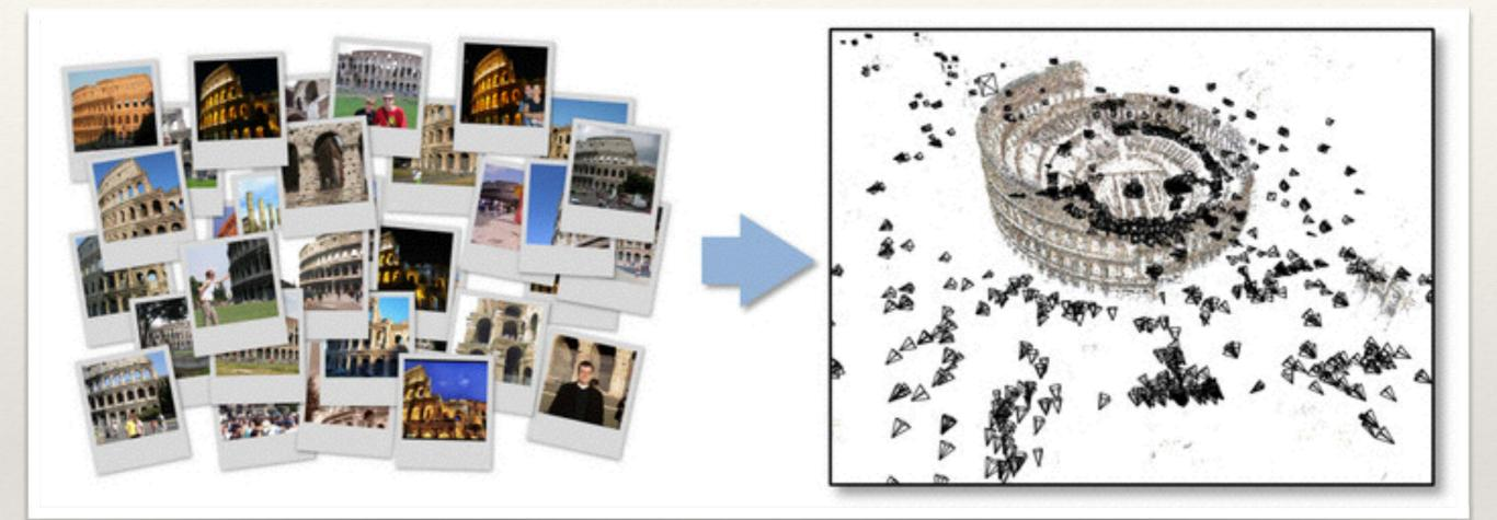
Multiple images can be used to jointly infer 3D structure, and the camera pose and intrinsics of each camera
